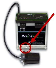
The Gateway serial number which is located on the mounting bracket of the device or on the inside panel of the enclosure is also required to be referenced on the Service Activation Form.
